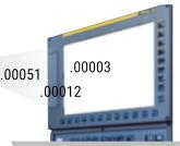
AutoComp calculates and updates offsets in the CNC control
